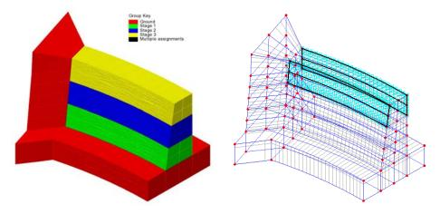
The temperatures and stresses for each time step for each construction stage can be obtained:
